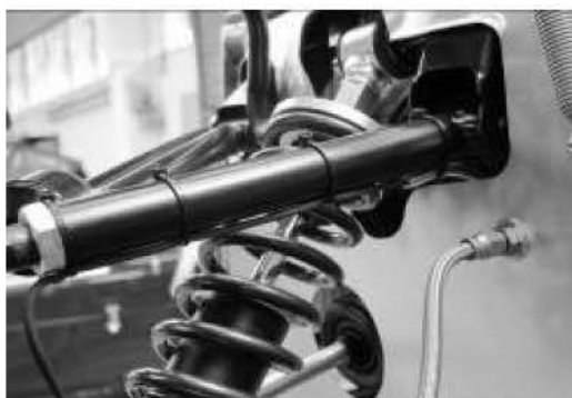
Headlight Wiring/Routing Picture 4
