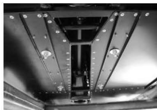
Step 18: Check seat bolts come through nyloc nuts.
