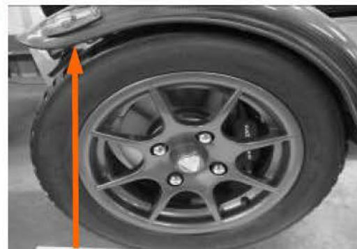
Step 20: Front wing leading edge must be over wheel.
